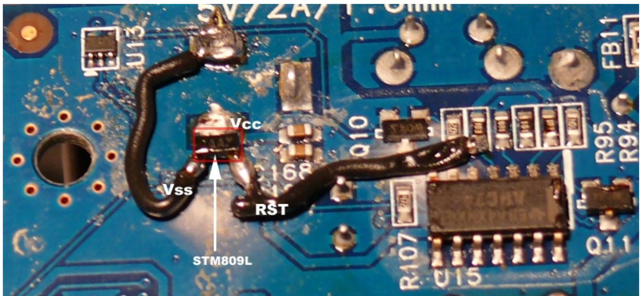
**STEP 5:** Done. Put it all together again. When you now attach the power plug to the NSLU2 it should immediately boot. Please try if the power-on/off button is still working as expected. Having passed these tests you now have the feature "auto reboot after power failure" implemented on your NSLU2.
